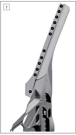
Drill out welding spots and remove the body side inner reinforcement and the side inner lower reinforcement. 3.
