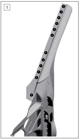
3. Drill out welding spots and remove the body side inner reinforcement and the side inner lower reinforcement.
