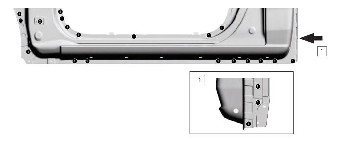
Install the side sill outer panel to vehicle body and cut in stacked condition. 3.
