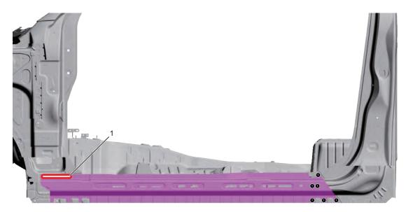
1. When heating around adhesive application portion to detach adhesive, be sure that temperature of said portion does not reach 170 °C (338 °F).
