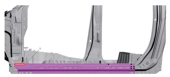
1. When heating around adhesive application portion to detach adhesive, be sure that temperature of said portion does not reach 170  $^{\circ}$ C (338  $^{\circ}$ F).
