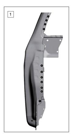
3. Drill out welding spots and separate the rear pillar inner lower panel.
