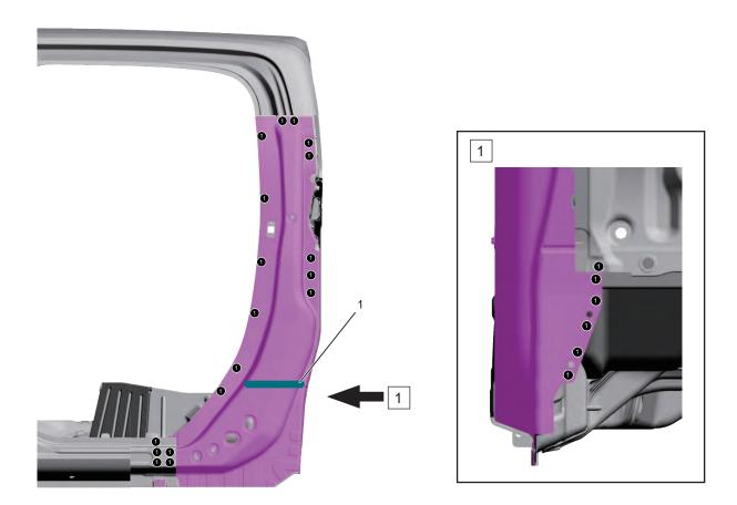
When heating around formed material application portion to detach formed material, be sure that temperature of said portion does not reach 170 °C (338 °F).
