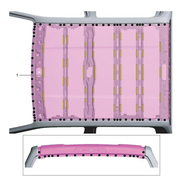
When heating around sealer application portion to detach body sealer, be sure that temperature of said portion does not reach 170 °C (338 °F).
