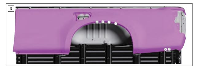
10. Tighten the 6 bolts to specified torque. Tightening torque 13N\*m {1.3 kgf-m}
