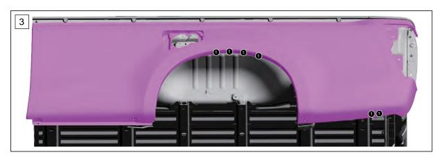
3. Drill out welding spots and remove the rear body front filler.
