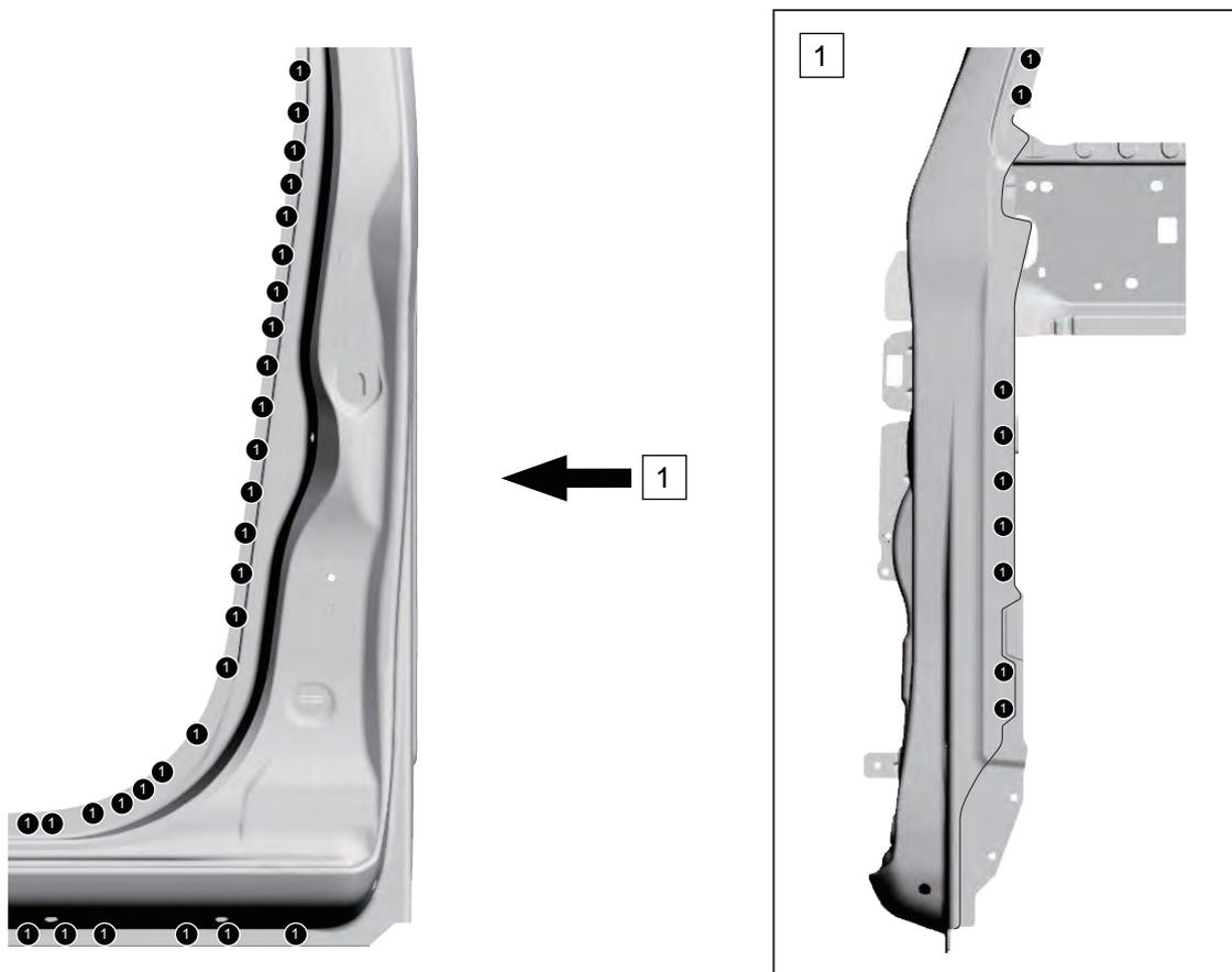
3. Install the front pillar outer panel to vehicle body and cut in stacked condition.
