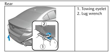
4) Attach a rope to the eyelet.
