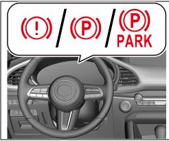
When the parking brake is applied with the power switch switched ON, any of the indicator/warning lights shown in the figure turn on.
