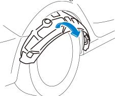
2) Insert a hand from inside the tire housing and pull the charge connector lock manual release lever in the release direction shown in the figure.
