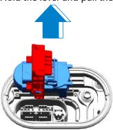
➤ After removing the service plug, leave it for 10 min.
