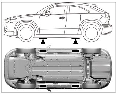
Support the vehicle at 4 points using the vehicle support positions shown in the rescue sheets for each vehicle model.
