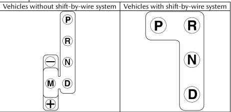
For vehicles with an automatic transmission, shift the selector lever to the P position so that the vehicle does not move. The condition in which the selector lever is in the P position can be checked by the indication in the instrument cluster while the power switch is switched ON.
