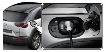
The charge port has a lock function to prevent the charge connector from being unplugged due to vibration or mischievous behavior during charging.
