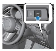
(2) Unlocking using electric trunk lid opener
